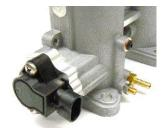
Install the TPS sensor using the included screws. Sensor can be mounted pointing inward or outward.
