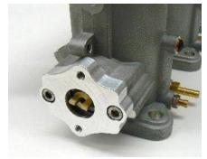
Install the TPS Adapter using the included screws.
