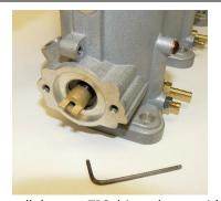
Install the new TPS drive adapter with included screw and Loctite.
