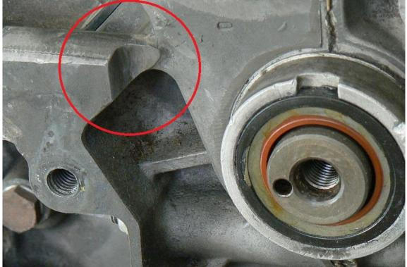
2. Remove the distributor. Apply oil to the distributor plug "O"-ring and the distributor hole. Insert the plug into the hole to the shoulder. Torque the center bolt to 14 ft/lb.
